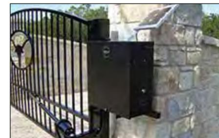
For people living in rural areas, a swinging solar-powered gate can be very convenient, eliminating the need to get out of the vehicle twice — once to open the gate and again to close it.
