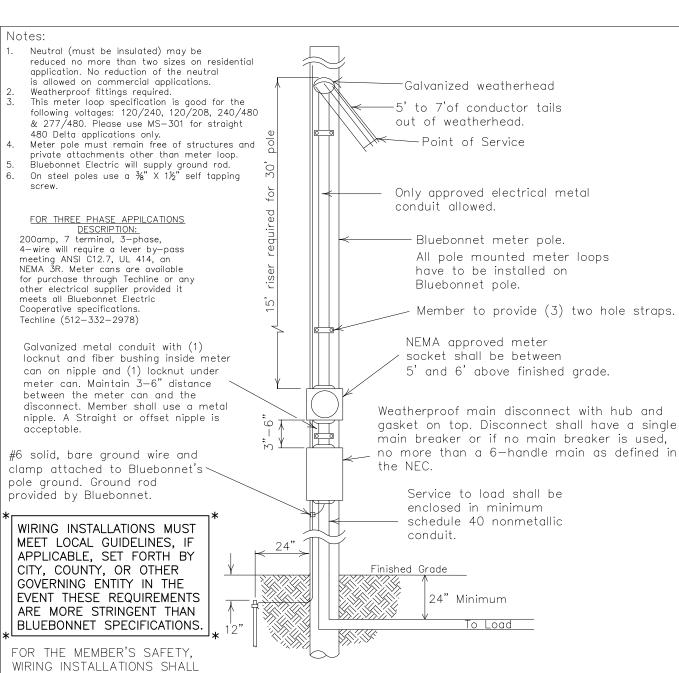
WIRING INSTALLATIONS SHALL CONFORM TO THE REQUIREMENTS OF THE NEC, TDLR AND NESC.
